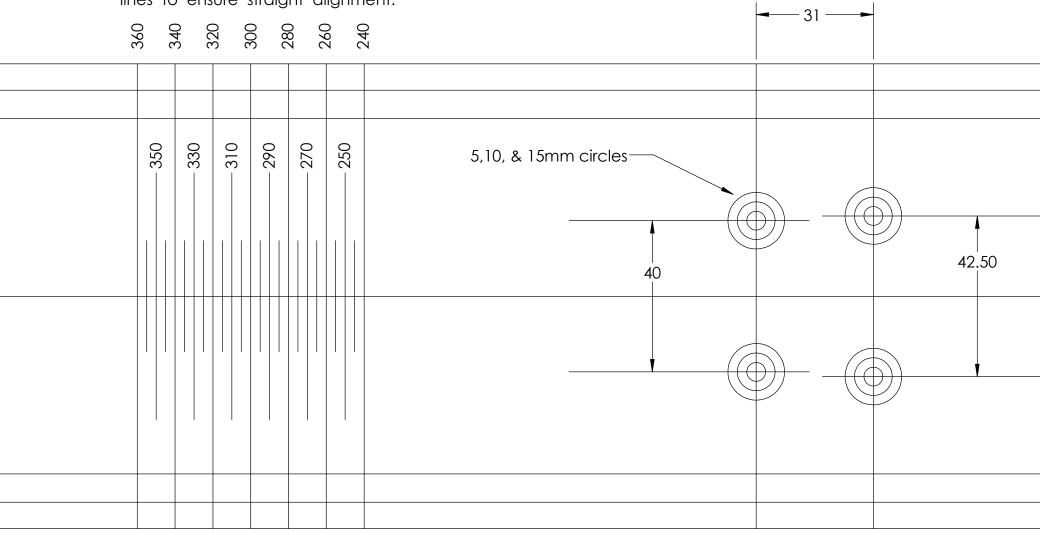
Reccomended to test mount for your boot on a 2 x 4 before drilling ski. Check printer scaling for labeled dimensions (mm)
